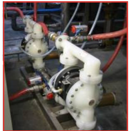
2 thickener transfer pumps pump the stock paste from holding tank to dye mixing tanks.
