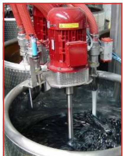
2 thickener transfer pumps pump the stock paste from holding tank to dye mixing tanks.
