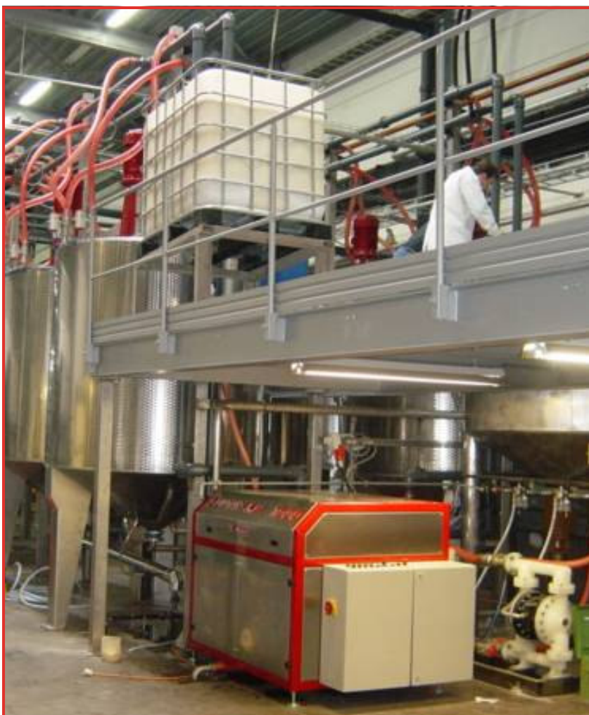
Typical layout of a thickener preparation system for a ChromoJet print line (6000 kg/hour)
